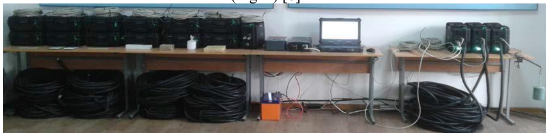
Figure 1. Tenso intelligent deformation and force monitoring system for analyzing loads in engineering structures
